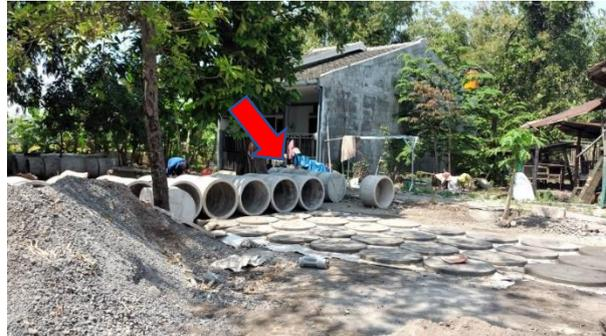
**Gambar 4.** Buis Beton Bahan Baku Septic Tank (Panah)
